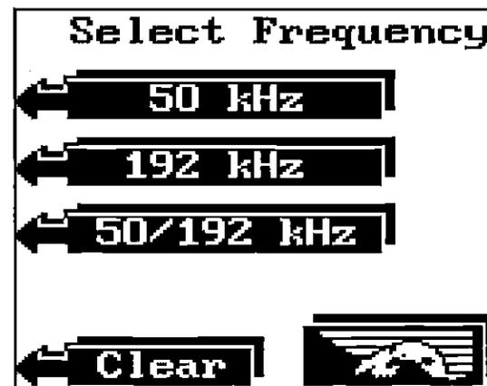
Now press the key adjacent to the desired frequency, either 50 kHz, 192 kHz, or both 50 and 192 kHz-split screen operation. The unit will begin scrolling echoes across the display.
